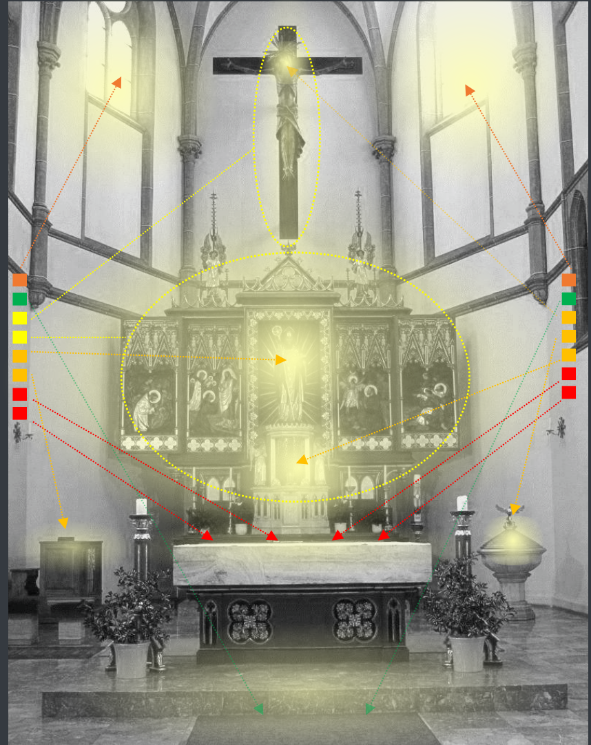
Oval Wide Flood LED 19,6W (Lichtquelle), 2700K, 1501lm, CRI 92
